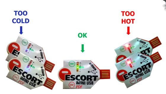
Now with expanded alarm thresholds, the user will be able to see a warning of temperature variances using the low and high settings as well as catastrophic levels with low low and high high settings, ensuring safe transport of perishable cargo.
