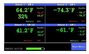
The picture above is of one fourth of the current status display showing the current conditions for one of the four sensors and the maximum and minimum temperature recorded. The current battery charge for the sensor is also displayed.
